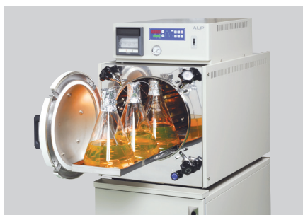
1. Lower tray : Accommodates 2 or 3 pcs. (model L) of Erlenmeyer flask 5 litres
