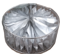
Non-stand-up pouch (Vertical placement) (180mm×140mm×20mm) 32 pcs./basket Total 96 pcs./operation
