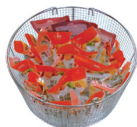
Stand-up pouch (180mm×140mm×30mm) 20 pcs./basket Total 60 pcs./operation
