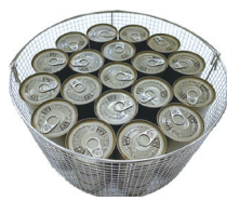
Steel can (φ75mm×110) 18 pcs./basket Total 54 pcs./operation
